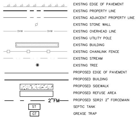
EXISTING STONE WALL EXISTING UTILITY POLE EXISTING BUILDING EXISTING STREAM EXISTING TREE \_\_\_\_ PROPOSED EDGE OF PAVEMENT PROPOSED BUILDING PROPOSED SIDEWALK PROPOSED REFUSE AREA SEPTIC TANK GREASE TRAP
