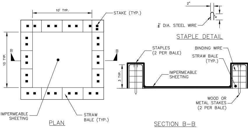
CONCRETE WASHOUT AREA WITH STRAW BALES NOT TO SCALE
