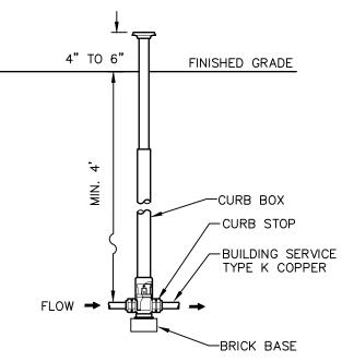
CURB STOP TO BE MUELLER H15200, OR EQUAL CURB BOX TO BE MUELLER H10306 WITH ROD, OR EQUAL CURB STOP DETAIL NOT TO SCALE
