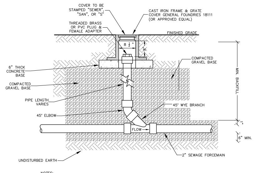
1. CLEANOUT LOCATED IN A ROAD, DRIVEWAY OR PARKING AREA SHALL REQUIRE A CAMBELL FOUNDRY #4164 CAST IRON FRAME AND COVER. (OR APPROVED EQUAL).
