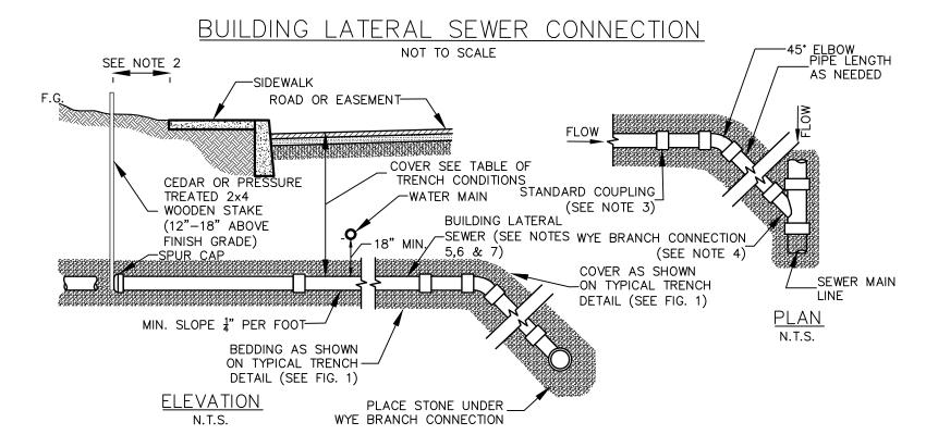
SANITARY SEWER SPECIFICATIONS (FOR BUILDING LATERAL
